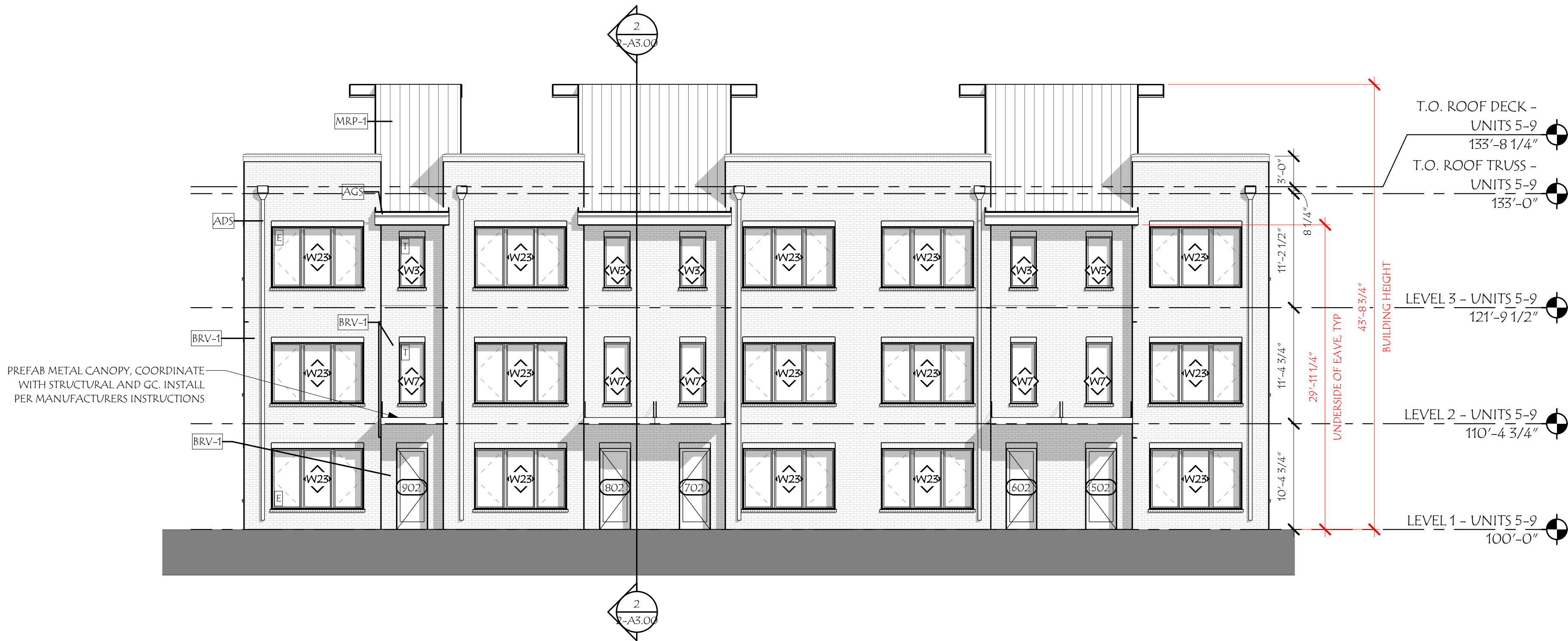
2 NORTH ELEVATION - UNITS 5-9 SCALE: 1/8" = 1'-0"
