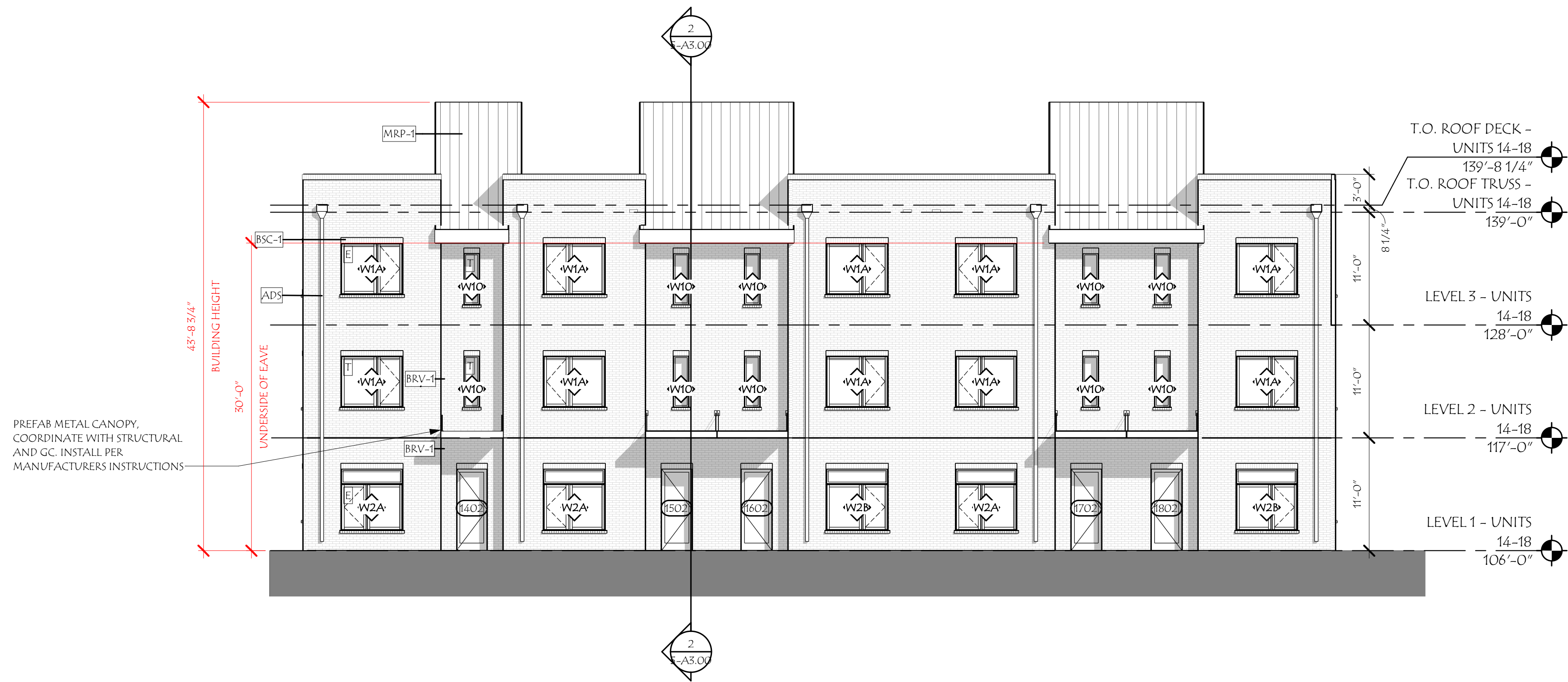
2 SOUTH ELEVATION - UNITS 14-18 SCALE: 1/8" = 1'-0"
