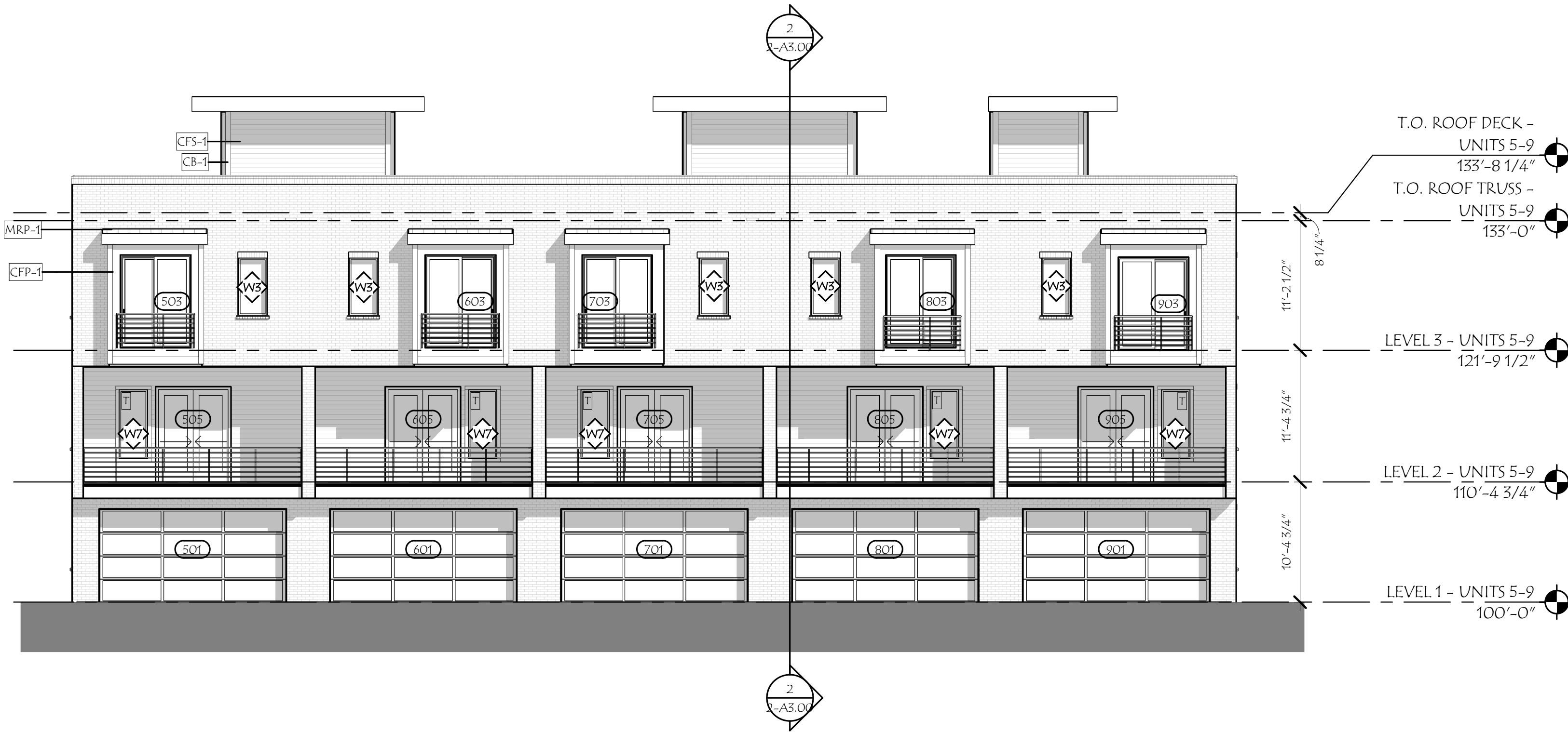
1 SOUTH ELEVATION - UNITS 5-9 SCALE: 1/8" = 1'-0"
